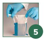
Fold both wire ends onto the bag to provide air-tight and leak-proof closure
