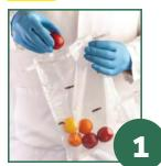
Insert the solid sample of the printed side if the FILTRA-BAG
